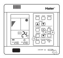
Before using TIMER function, calibrate the clock first.
